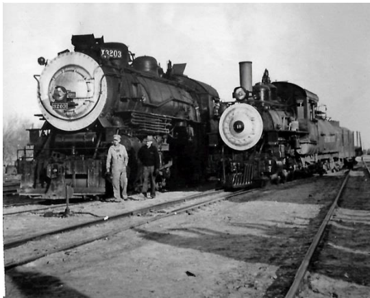
Exhibit 12 Standard Gauge (left) vs. Narrow Gauge
